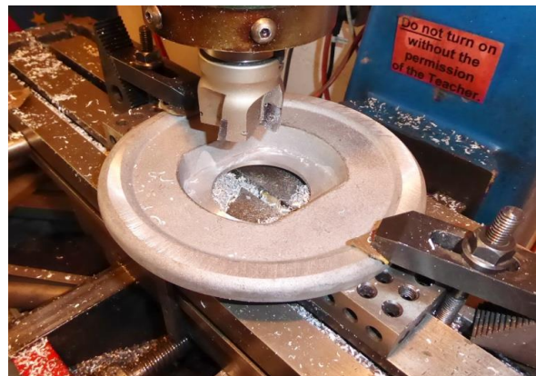
Fig 4 - Truing-up the inner face of the recess
